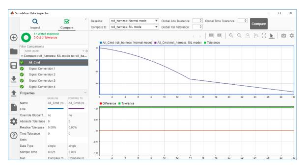
The Simulation Data Inspector shows that the normal mode and SIL mode results match. Comparing the results of normal mode simulation with SIL and PIL simulations can help you verify that the generated application performs as expected.
