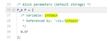
The code that you generate from the model stores the parameter object in memory. Because you left the default storage class settings in the Code Mapping Editor for category **Model parameters** set to **Default**, the code generator determines the storage format, for example, as fields of structures.
