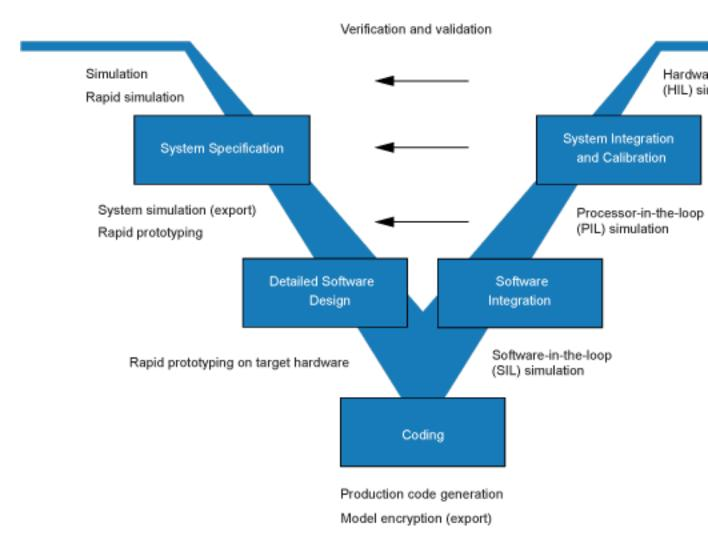
Depending on your application and its role in the process, you might focus on one or more of the steps called out in the V-model or repeat steps at several stages of the V-model. Code generation technology and related products provide tooling that you can apply to the V-model for system development. For more information about how you can apply MathWorks code generation technology and related products to the V-model process, see:
