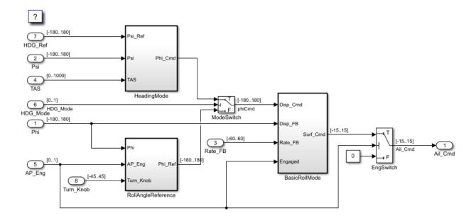
This model implements a basic roll axis autopilot algorithm, which controls the aileron position of an aircraft.
